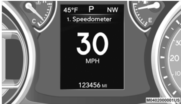
3.5 Inch Instrument Cluster Display Location
