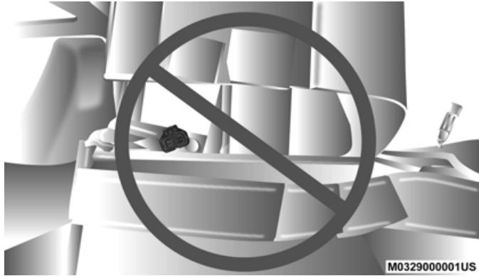
Incorrect Placement Of Wire Harness
