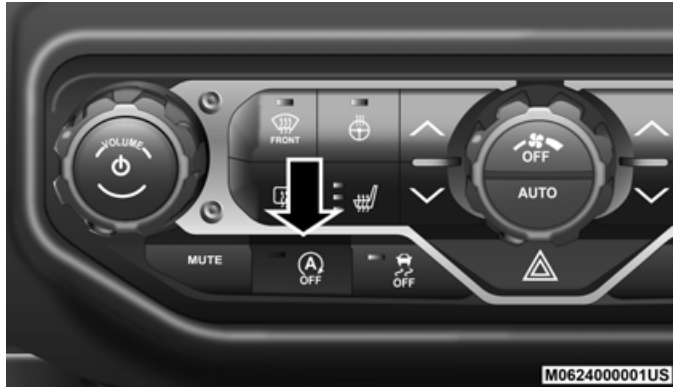
STOP/START Off Switch
